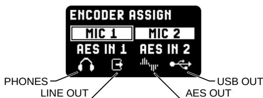
In this screenshot, the encoder is assigned to both MIC 1 and MIC 2 input gain. Bottom icons represent output assignments (only stereo gain is available in this case).
