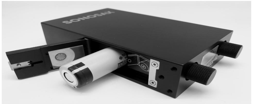
Insert the battery in the SX-M2D2 with the '+' polarity visible.
