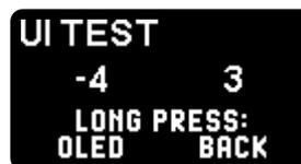
The two numbers in the middle of the screen are counters. Use them to test the rotary encoders. Rotating the encoder clockwise increases the counter and counterclockwise decreases the counter. An encoder short press highlights its counter.
