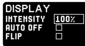
INTENSITY modifies the display brightness. The range of values is 0 to 100% with 10% steps. A 0% value corresponds to the minimal display intensity (pixels are still visible).
