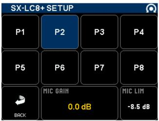
The presets are labeled P1 to P8. To store the current configuration, press and hold the corresponding button until a confirmation message appears. To recall a preset, short press the corresponding button.
