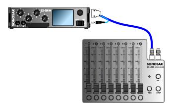
On the SX-R4+ side, a 3M MDR 26-pin connects with the SX-LC8+. The female TA3 connector is the SX-LC8+ slate/com microphone output, it is intended to be connected to the SX-R4+ AUX AES input.
