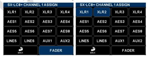
On the left, the fader is assigned as a mixing fader. To operate with mixing fader, they must be assigned to mix tracks in the MIX menu.
