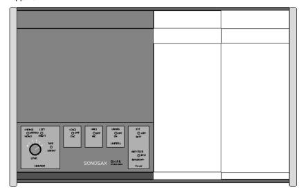
MONITOR In this area you find all the necessary switches and buttons for the headphone monitoring.
