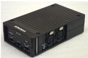
2 channels microphone pre-amplifier with 48V Phantom
