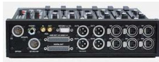
An 8 ways A/D converter is also available as an option. It converts the 6 direct outputs of the channels and the main mix 1&2 onto four AES/EBU transformer balanced outputs.
