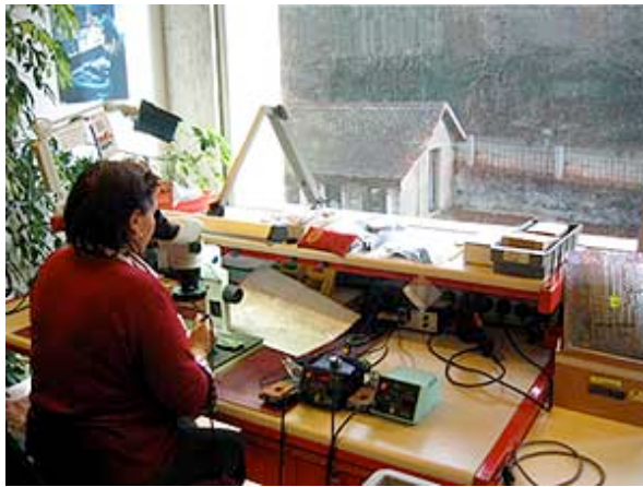
Visual inspection of all circuit boards happens here.
