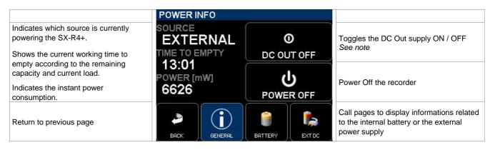
**NOTE :** The voltage on the Hirose 4 pin connector [DC OUT] depends on the power source of the SX-R4+ : - if the recorder is powered from the internal battery the DC Out voltage is internally regulated to 12V - if externally powered, the DC Out voltage is directly derived for the Hirose 4 pin [DC IN] connector.
