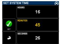
[SYSTEM TIME] and [SYSTEM TIME] are set in a similar manner; select a field then use the encoder wheel to set the value. Validate the selection with the key.
