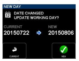
If the working day has changed while powering up the unit, the system asks to confirm the date of the new working day. This allows keeping the date of the current working days if the on going production works is passing across midnight.
