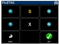
[FILETAG] is a unique identifier automatically generating the audio files name. The first 2 characters can be modified by the user, which might be useful to identify the recorder unit when multiple recorders are used on the same production.
