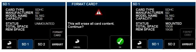
Insert a SD card in a slot, then press the Format Card
