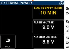
Set the Alarm "Time to Empty"; available only if a SMBus battery is connected to the [DC IN] connector. See note above
