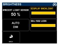
[LIGHT SENSOR] indicates the ambient light intensity
